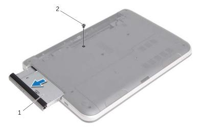
optical-drive assembly screw
